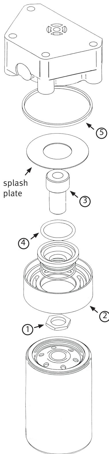
To compensate for the variations in Filter Head tolerances the Spin On consists of three parts Spin On Inner and Outer and an o ring. The variations in tolerances are taken up by the Spin On Outer sliding over the Spin On Inner. The integrity of the seal between the Inner and Outer is maintained by an o ring.
