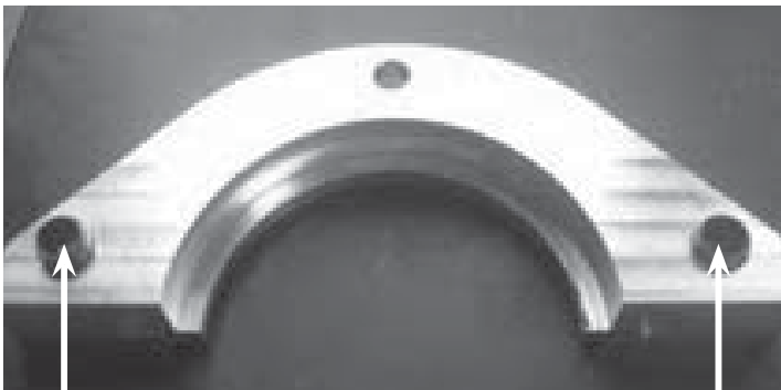
3. Install the dowel pins into the top half of the seal housing.
