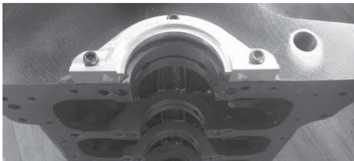
5. Install the top half of the new seal housing to the back of the block. Use Loctite on the threads of all three of the 5/16” allen head bolts.
