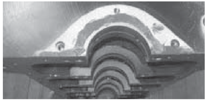
4. Use a light coat of ATV to seal the housing to the block.
