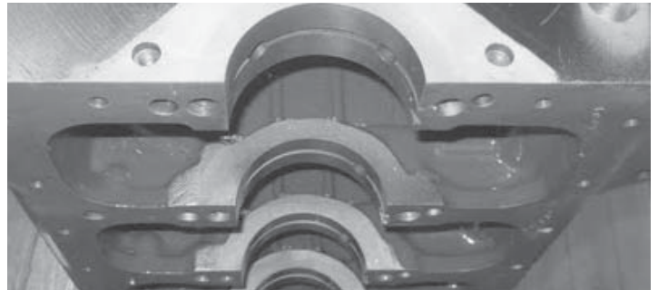
2. Rear of block must be clean at seal area!
