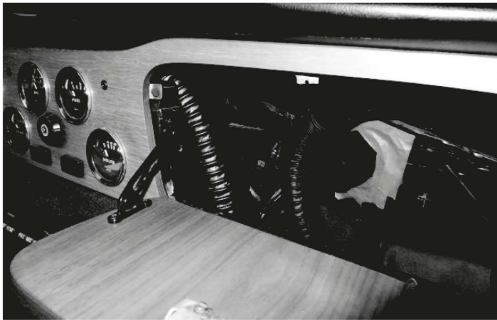
Glove box removed showing the vent hose and the longer defroster hose.
