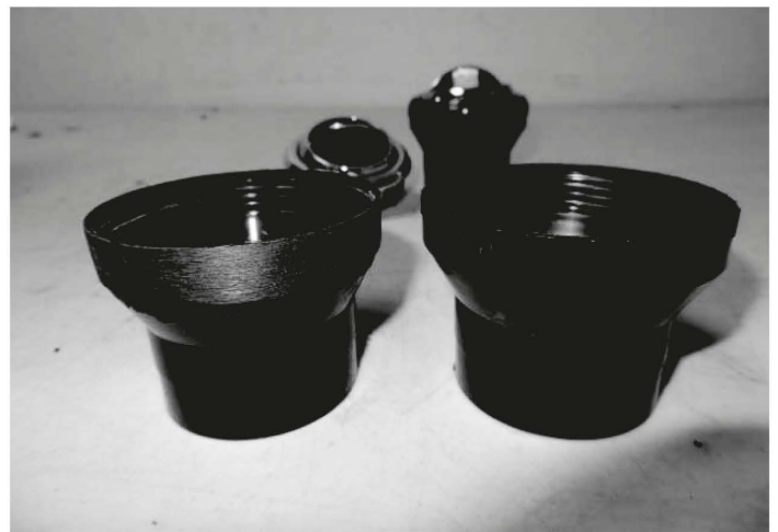
The round vent collar on the left is sanded down to fit into place.
