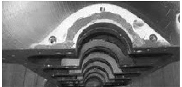
4. Use a light coat of ATV to seal the housing to the block.
