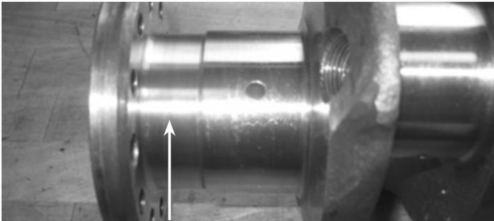
1. The seal area at the rear of the crankshaft needs to be machined to 66.85 mm (2.632").
