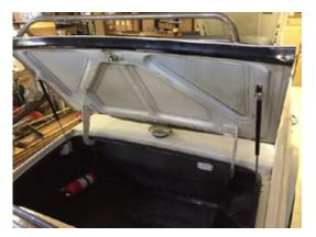
15. Finally, attach the 4 locking springs to the strut end-fittings. These will prevent the struts from detaching if ever they are bumped. Insert the wire fully and then rotate until it snaps onto the end-fitting collar, thus locking the ball stud inside the end-fitting. Some are blind. Start with the top right hand one since it is visible/easiest.
