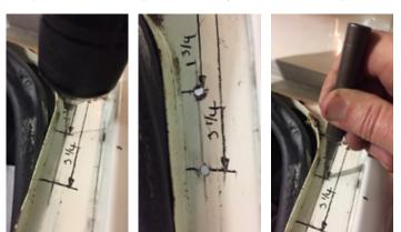
9. Fasten the lower bracket using the machine screws and Kep nuts; see photos. Replace the boot lid gasket.
