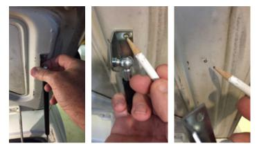
12. Drill this point with a 7/64" drill bit. Note: Use a stop collar on your bit, so you don't accidentally plunge through and dent your boot lid outer surface.
