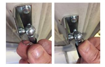
16. Periodically use a non petroleum-based lubricant on the struts and on your trunk gasket so their touching does not become abrasive. Dry Silicone Spray is ideal; available at ACE hardware stores.
