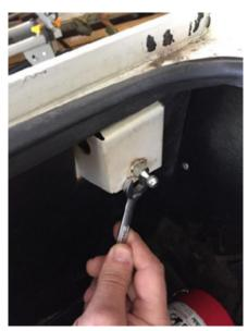
3. Install the upper (boot lid) ball stud without any washer at all. It is best to use a drop of thread lock so this never vibrates loose. Do not over tighten!
