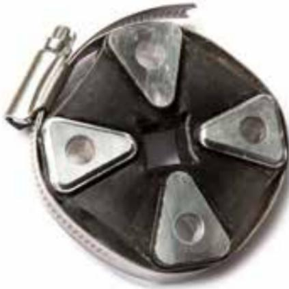
Pretensioned in this way, the bolts of the flanges can easily be guided through the bushes of the joint discs and mounted.
